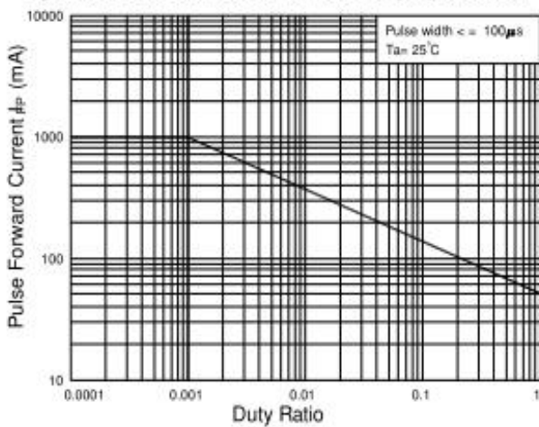
Figure 5. Pulse Forward Current vs. Duty Cycle Ratio
